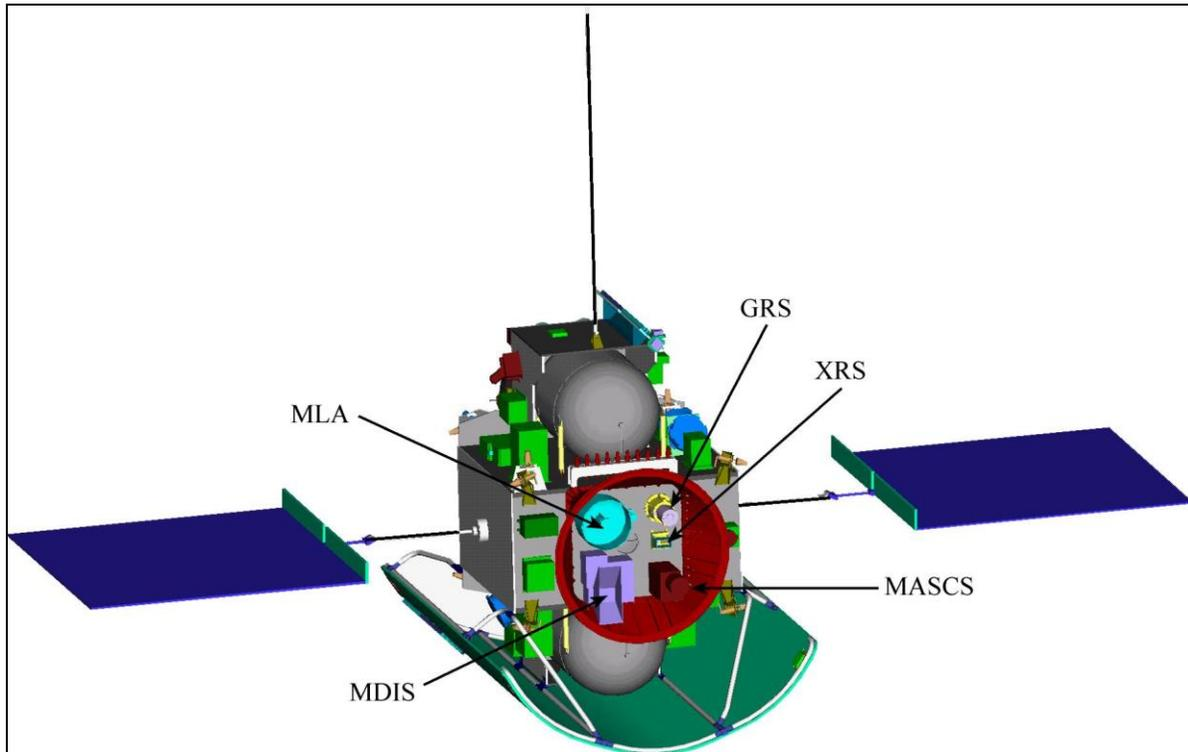
Figure 4: MESSENGER instrument deck showing instrument accommodation.
