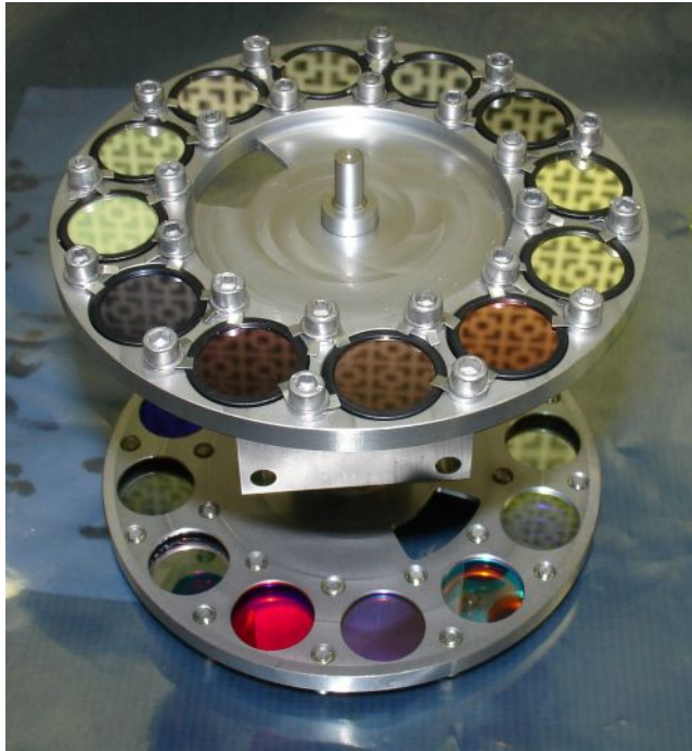
Figure J-6. The FM SSI Filter Wheel just after assembly. Each wheel is for one eye. The pattern in the filters is the reflection of the screen on the back of the flow bench.
