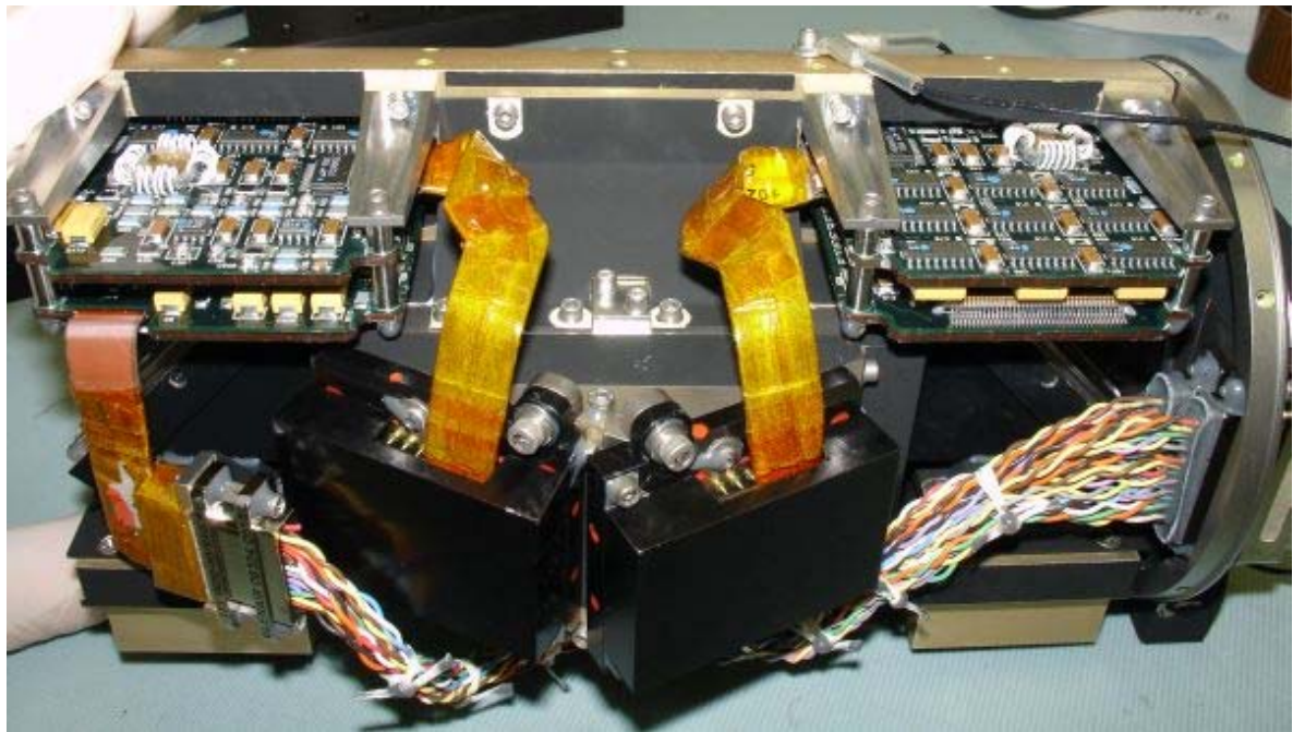
Figure J-4. Image of the camera head without the cover showing the two MER CCD's and two sets of MER electronics. The CCD's are under the two black rectangular pin covers at the end of the gold flex cables which connect the CCD's to their electronics.
