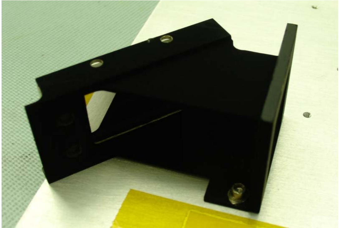
Figure J-9. The right fold mirror and mount assembly. Most of the surfaces of the mount are finished with the Martin Black Process.
