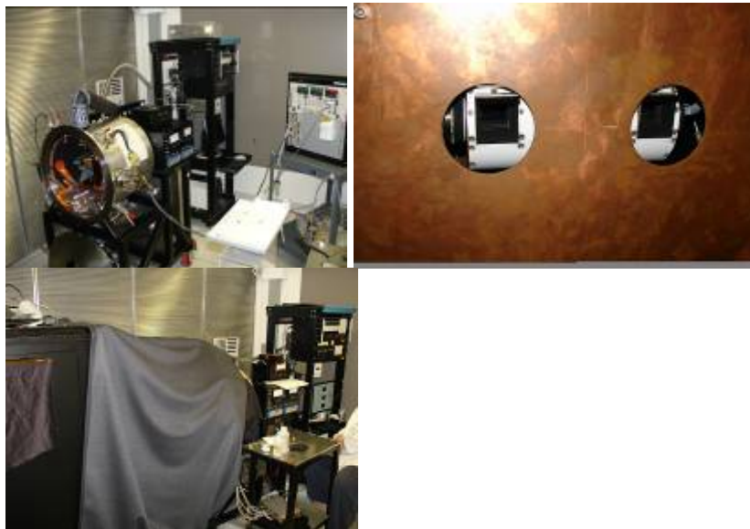
Figure. C-2 Open TVC chamber (left), SSI looking through the cold baffle ports in the TVC (center) and full responsivity setup with the TVC draped to the Black Box where the Spectralon resides.
