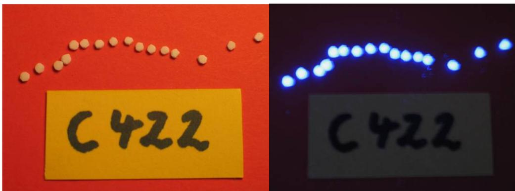
Figure 2. BAM batch C422 seen in VIS (left image) and UV (254 nm, right image). Tablet #2 and #5 (from left to right) were selected as FS1 and FM1, respectively
