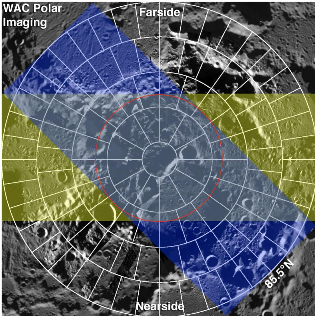
**Figure 3.1.3** – Two WAC swaths (one shown in blue and one shown in yellow) taken 3.5 days apart at the North Pole. Every orbit has repeat coverage between 88° and 90° latitude.
