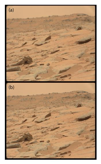
Figure 28. Example results from a special eight-image z-stack M-100 image test conducted on Curiosity sol 193 with sequence mcam01026. (a) One of the eight images acquired of the scene, with focus set for the foreground. (b) The resulting focus-merged z-stack image calculated automatically in Mastcam flight software. Note the dramatic removal of depth-of-field effects, especially for the far ridge.
