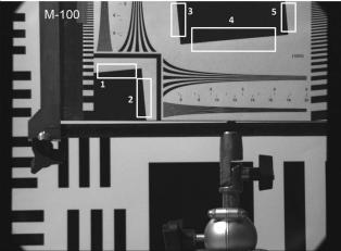
Figure 12. Example flight Mastcam (top) 34 mm and (bottom) 100 mm preflight calibration interpolated Green Bayer pixel images of the SVG Squares and Wedges pattern target [Imatest, 2015] used to assess the MTF performance of the flight cameras. Five regions of interest, numbered on each image, were analyzed.
