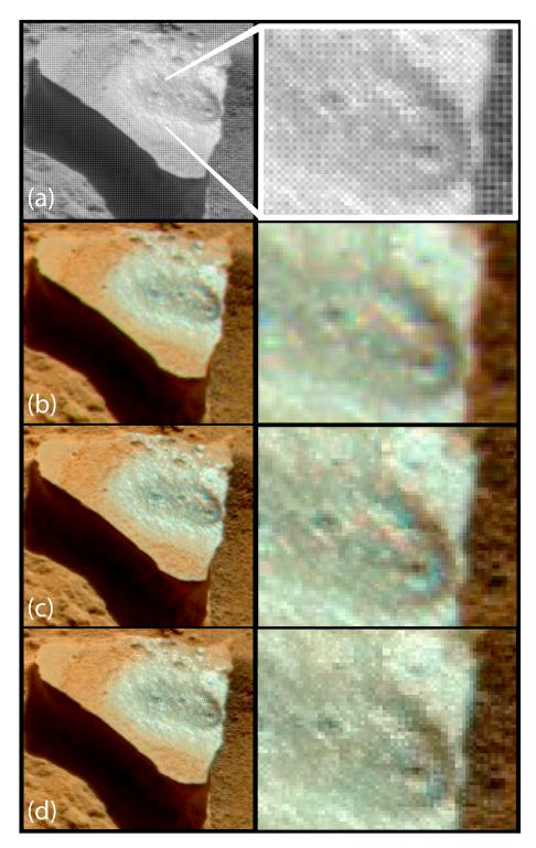
Figure 23. Comparison of (a) raw MSL Mastcam image showing the original Bayer filter pattern, versus application of (b) bilinear interpolation, (c) default Improved Linear Interpolation (ILI) or Malvar-He-Cutler, and (d) Directional Linear Minimum Mean Square-Error Estimation (DLMMSE), or Zhang-Wu, demosaicing algorithms. Portion of Mastcam M-100 image 0620MR0026570000401488C00\_DXXX, with zoomed insets on the right.
