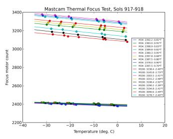
**Figure 17.** Dependence of focus motor count on Mastcam focal plane array temperature for the M-34 and M-100 Mastcams, based on six inflight mosaic sequences acquired on Mars on *Curiosity* sols 917 and 918.
