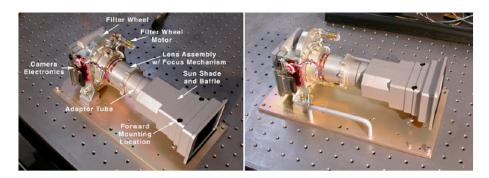
Figure 1. The Mastcam (left) M-34 camera head and (right) M-100 camera head. For scale, spacing of the optical table's bolt hole pattern is 1" (2.54 cm).
