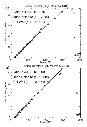
Figure 5. MSL/Mastcam (a) 34 mm and (b) 100 mm preflight CCD linearity, gain, and full well photon transfer curve data sets, with resulting CCD parameters derived using the methods of Janesick et al. [1987].
