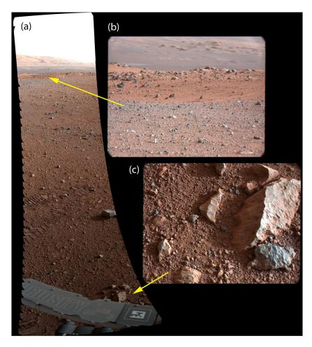
Figure 27. Images from the special 1 column × 34 row focus test mosaic acquired with the Mastcams on *Curiosity* sol 17. (a) Mosaic of 34 M-34 images acquired in the test, each acquired with 75% overlap relative to the previous one. (b) Example of one of the M-100 images from the mosaic with nearer, middle, and far ridges in the same scene. (c) Example of another M-100 image from the mosaic with near-field targets at a variety of distances.
