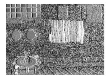
Figure 15. Band depth map at 865 nm (relative to continuum wavelengths at 751 nm and 1012 nm) generated from a portion of the Mastcam M-34 preflight geologic target multispectral imaging campaign (Figure 14). This spectral parameter is sensitive to the presence of crystalline hematite and indeed highlights the hematite-bearing color chip on the lower left of the Mastcam calibration target and the hematitebearing layers in the Banded Iron Formation geologic sample.
