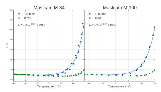
Figure 8. Zero-exposure bias signal (green data points) and 1000 ms dark current (blue data points) data for the (left) M-34 and (right) M-100 Mastcam CCDs, as a function of Focal Plane Array (FPA) temperature. Fits to the dark current data show the functional form of the Mastcam dark current model, in DN/s.
