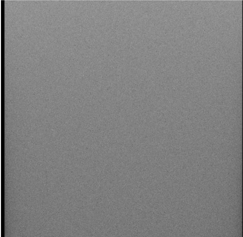
Figure 3.2.1n. Dark-current-corrected image (same image as Fig. 3.2.1j). The complete set of model dark-current components (Reference Pixel Variation, Zero-Exposure Variation, and Active-Area Variation) has been subtracted. The residual mean for this image is \sim 20 DN compared to the original raw mean of \sim 1500 DN. The standard deviation has been reduced from \sim 121 DN to \sim 22 DN.
