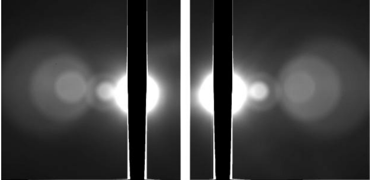
Figure 3.2.9c. Typical ghost images in MI serial # 105 images, corrected for transfer smear and stretched hard to show ghosts. Maximum ghost intensity \sim 0.02\% . (left) Image 020718082943, yaw +6.4^\circ . (right) Image 020718084958, yaw -7.8^\circ .
