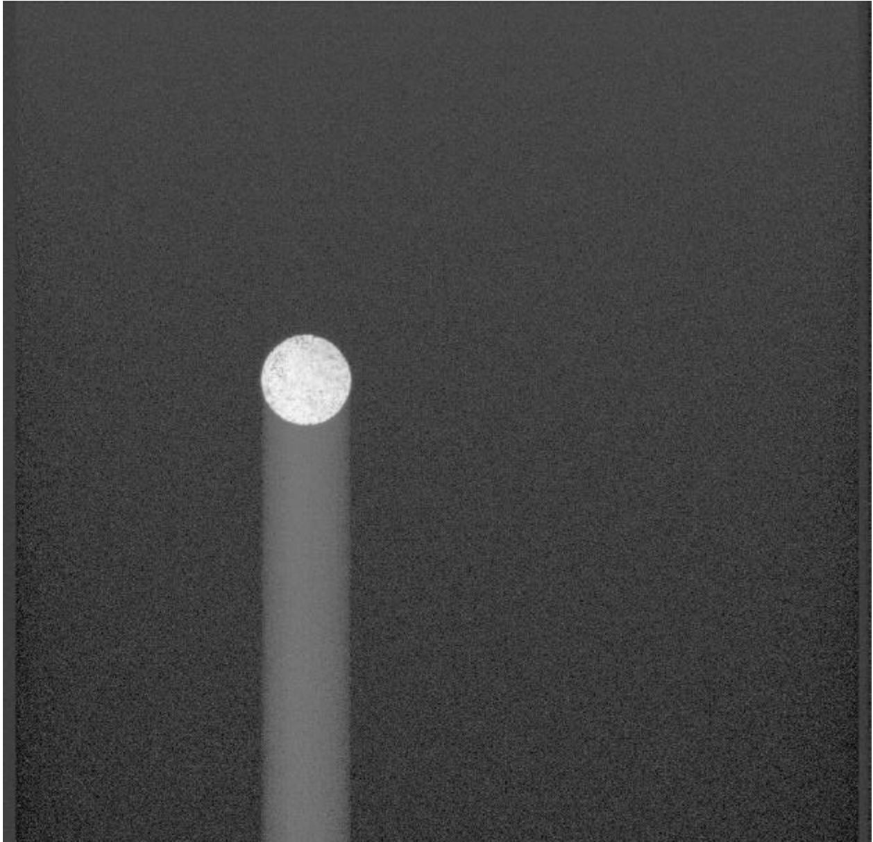
Figure 3.2.6a. MI serial # 105 image of fiber (020718092113_0000102) taken under ambient conditions with exposure time = 10.24 msec. Average zero-second dark frame has been subtracted to remove dark current accumulated during readout. Image transfer direction is toward top; note transfer smear below fiber image.
