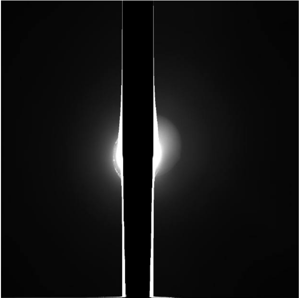
Figure 3.2.9b. Worst-case ghost image for MI serial # 105 (020718084631). Zero-exposure “shutter” frame (also saturated) was subtracted from the raw image, resulting in the column of pixels with DN = 0 at center. Hard linear stretch used to show ghost image.
