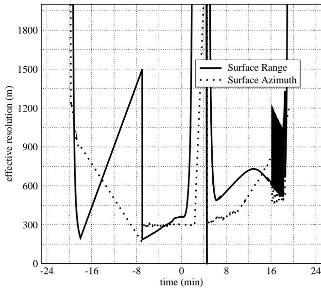
Figure 4: SAR projected range and azimuth resolution. These values are computed from the IEB parameters and are not related to the pixel size in the BIDR file. The pixel size was selected to be always smaller than the real resolution.
