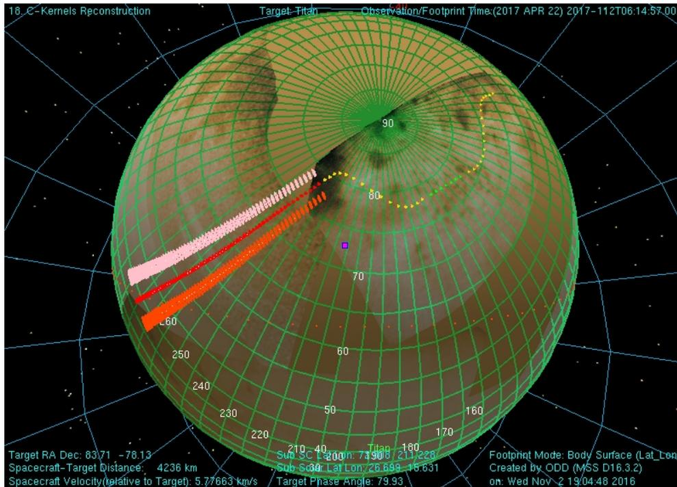
Figure 3: Beam 3 boresight (yellow triangles) during the close approach altimetry track and associated turns, and outbound SAR imaging swath (red and violet symbols) shown on Titan north polar map.
