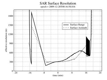
Figure 1: SAR projected range and azimuth resolution. These values are computed from the IEB parameters and are not related to the pixel size in the BIDR file. The pixel size was selected to be always smaller than the real resolution.
