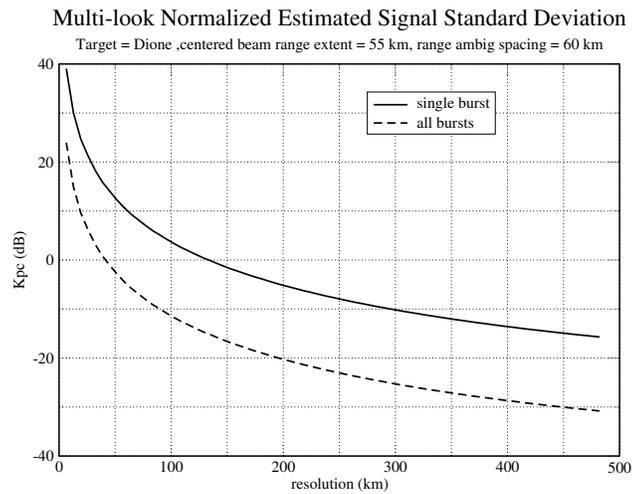
Figure 5: Div N: Normalized estimated signal standard deviation for a range/doppler cell as a function of resolution. Range/doppler resolution elements are both set equal to the specified resolution. Results are shown for a single burst, and for all the bursts in this division. Calculations are performed using the geometry at the start of the division. The presence of ambiguities are not shown.
