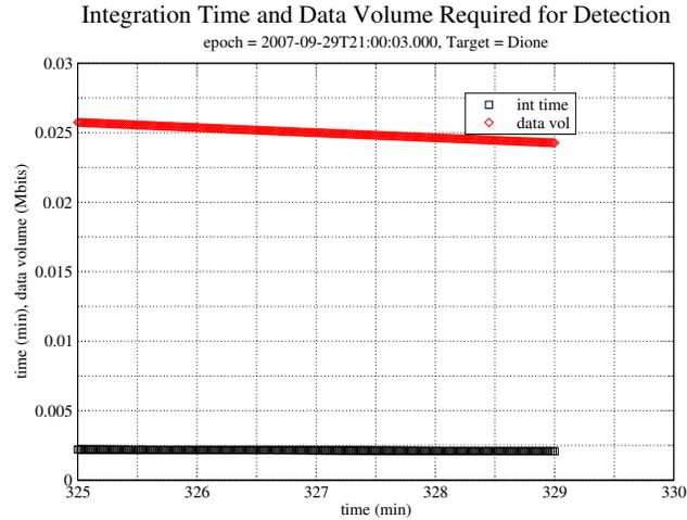
Figure 3: Scatterometry Div M: Detection integration time required for a single point detection using optimal chirp bandwidth
