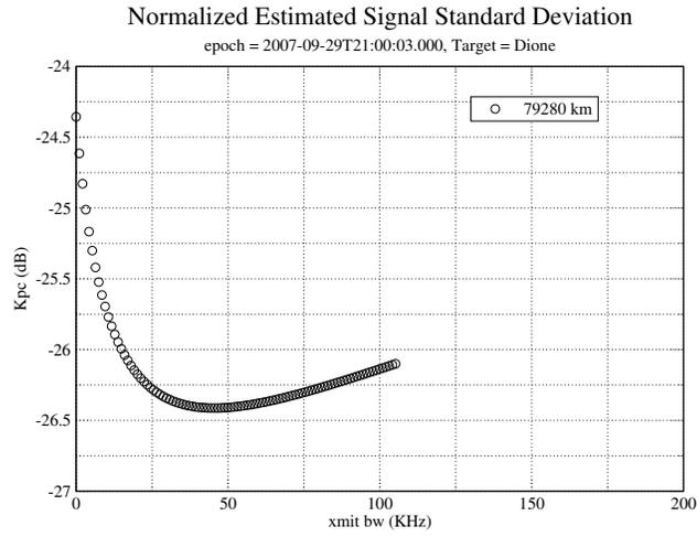
Figure 4: Div M: Normalized estimated signal standard deviation for a disk integrated observation using optimal chirp bandwidth and assuming all the bursts occur at minimum range, and 15 minutes away from minimum range.
