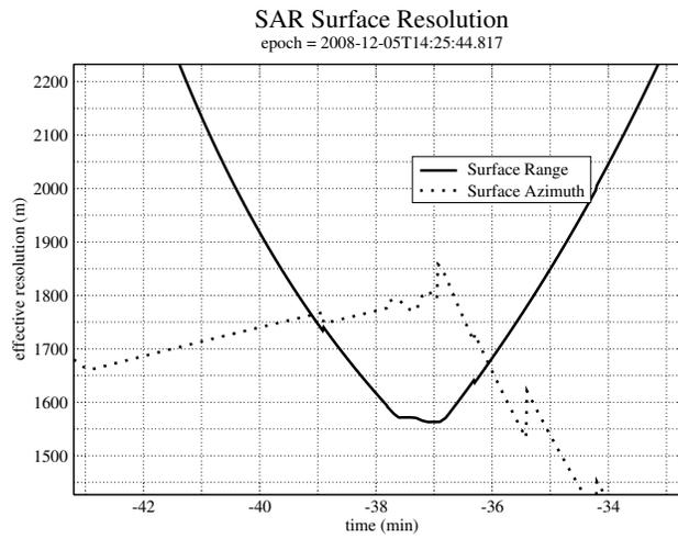
Figure 2: Inbound Scatterometer imaging projected range and azimuth resolution. These values are computed from the IEB parameters.
