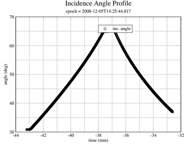
Figure 1: Incidence angle variation during Inbound scatterometer imaging.
