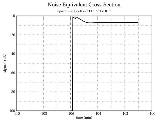
Figure 6: Div D: Noise equivalent  $\sigma_0$ . These values are computed from the IEB parameters.
