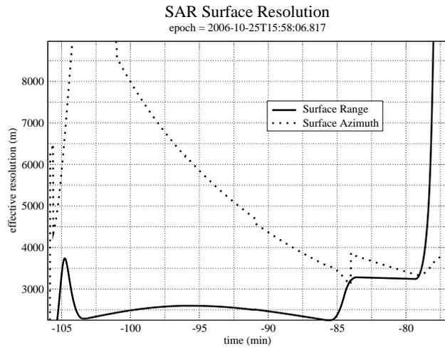
Figure 3: Div's D-I: Projected range and azimuth resolution. These values are computed from the IEB parameters.
