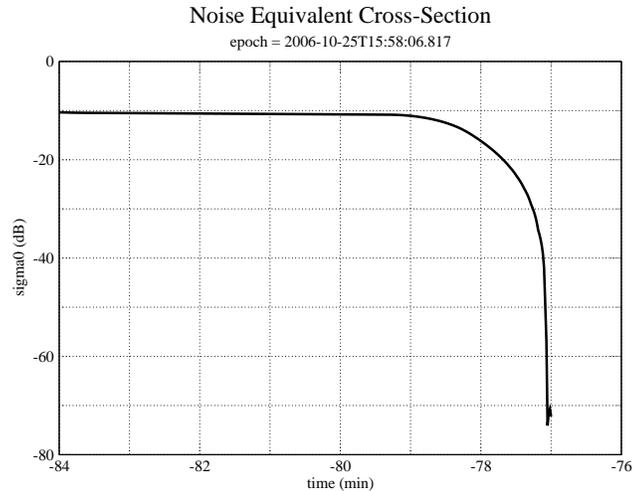
Figure 7: Div I: Noise equivalent  $\sigma_0$ . These values are computed from the IEB parameters.
