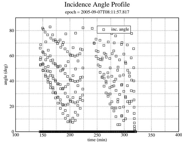
Figure 7: Incidence angle variation during radiometry/scatterometry scan
