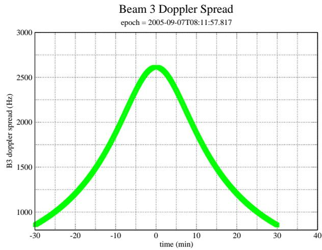
Figure 2: Nadir pointed B3 doppler spread during the time around c/a. Doppler spread is measured within the on-way 3 dB beam pattern.
