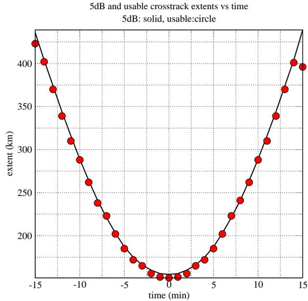
Figure 3: Usable cross track coverage predicted for the parameters in Div's C-E and the 950 km PRF and incidence angle profiles. Usable image area must have a signal to ambiguity ratio of at least 14 dB, a noise equivalent  $\sigma_0$  of at least -10 dB, and a one way antenna gain of at least -5 dB relative to the beam maximum gain. The large drop at the ends are due to the absence of beams 2 and 4 which are offset from beams 1, 3, and 5.
