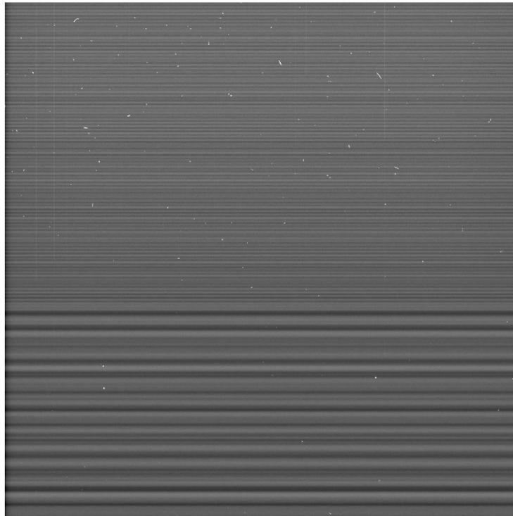
*Figure 8: Example of the 2 Hz horizontal banding pattern in a NAC dark image. This particular image was too large to fit completely in the image buffer during readout, resulting in a significant change in the readout rate half-way through. From Porco et. al. (2004).*
