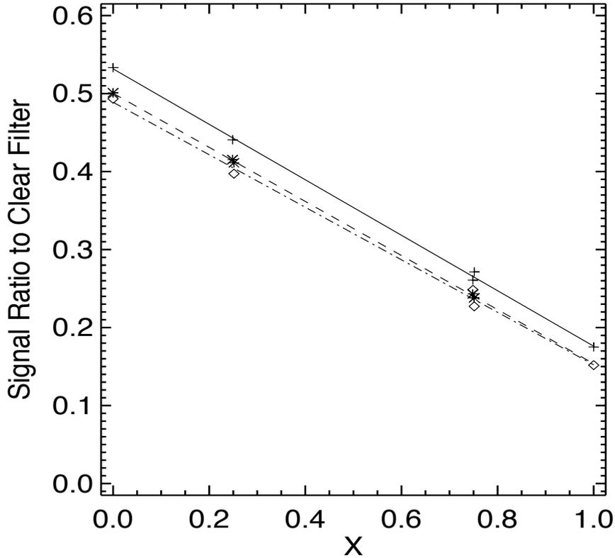
Figure 13: The ratio of the signal in each of three visible polarizers to the signal in the CLR filter (each paired with the BL2 filter) are shown as a function of  $x = \text{Cos}^2(\vartheta)$ . The measurements are shown as symbols for the three polarizers and the straight lines are linear fits to the measurements.
