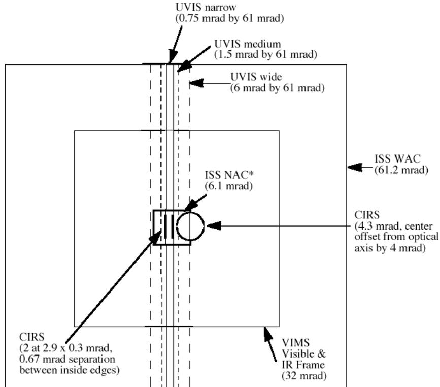
\*ISS NAC calibration shows offset by +0.822 mrad in X and -0.426 mrad from in Z from the -Y axis. Other instruments are shown in their nominal positions.
