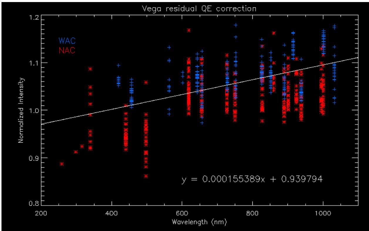
*Figure 16: Residual QE correction derived from Vega using the newly-derived correction factors. The fit line is applied to the QE correction function for both cameras, ensuring that the camera-to-camera ratio remains constant with filter.*
