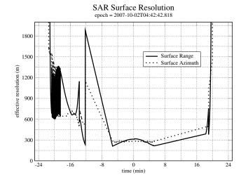
Figure 3: SAR projected range and azimuth resolution. These values are computed from the IEB parameters and are not related to the pixel size in the BIDR file. The pixel size was selected to be always smaller than the real resolution.
